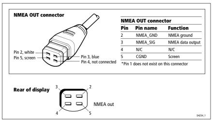
Figure 6-13: NMEA Output Connector
